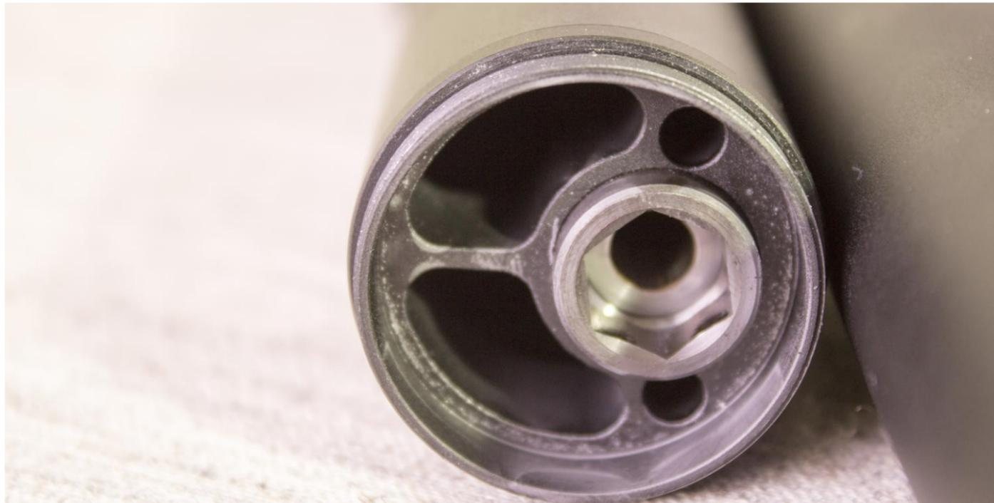
It is not recommended to completely disassemble the compression nut and clamping unit, as there is a possibility of losing fixing balls and springs.
