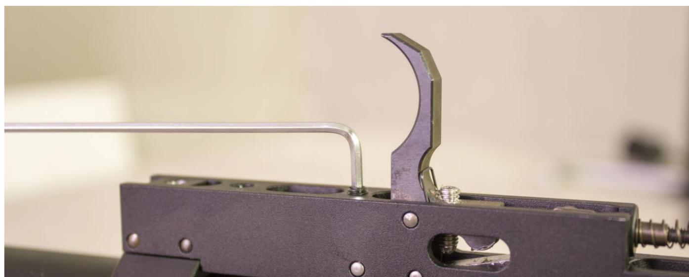
It is also possible to carry out this adjustment through the holes in the trigger guard without removing the bed.
