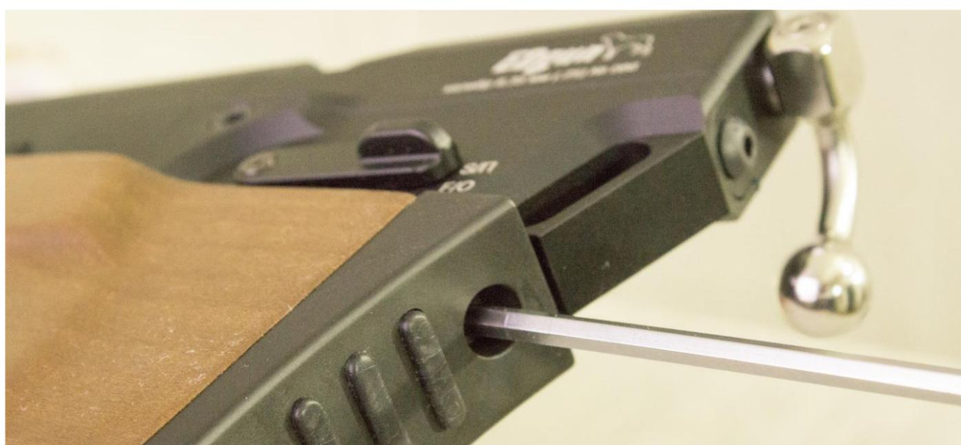
Remove the screw from the bottom of the trigger guard
