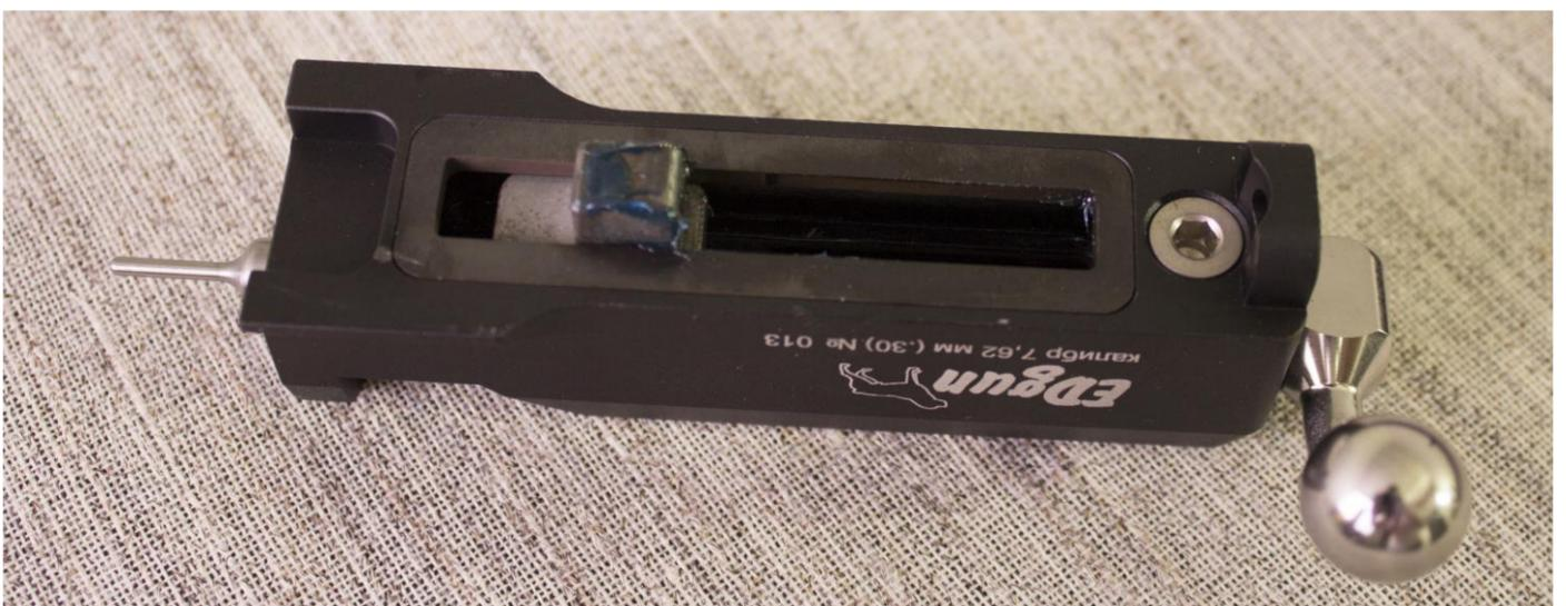
Note that the O-ring seal is located in the breech. Sometimes the the O-ring can fall out, sometimes it remains in the breech. Do not lose it. It the O-ring is missing you will feel a puff of air coming from the breech upon firing.
