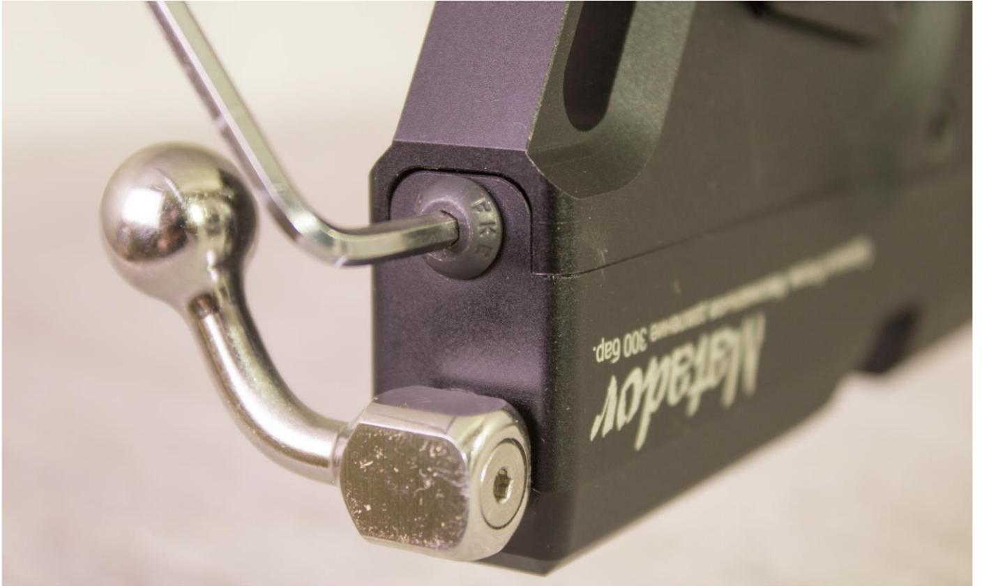
Pull out the bolt-frame assembly with the bolt.
